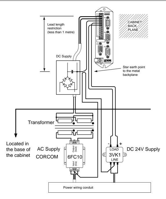
Figure 3-5. ViX EMC Installation
